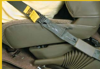
Belt tension and the force applied to occupants' chests may be limited by allowing webbing to tear (left) or spooling some webbing from the retractor (right). The issue is whether force limiters, whatever their mechanisms, protect people from injuries or allow them to occur.
